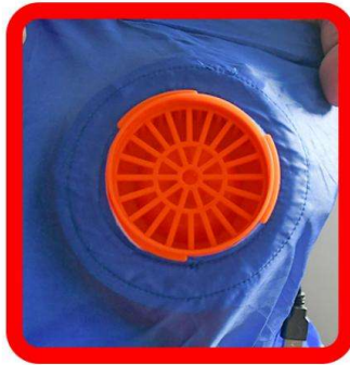
5. Put the blower in the round hole
