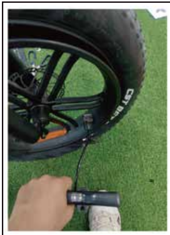
17. Fill the tires with air
