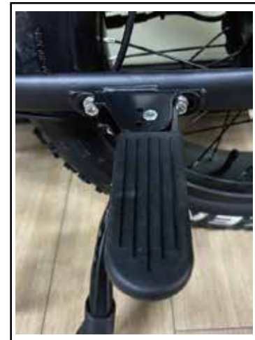
18. Install the pedals and tighten the screws
