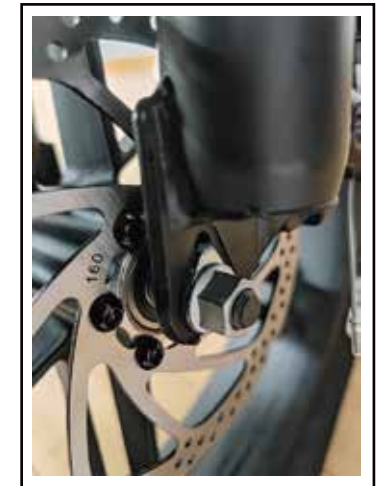
12. Install the wheels and pay attention to the order of the accessories
