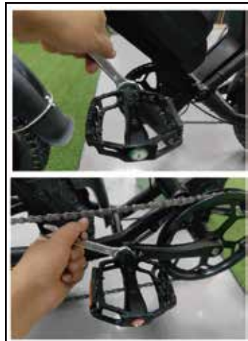
16. Install the pedal and tighten the screw
