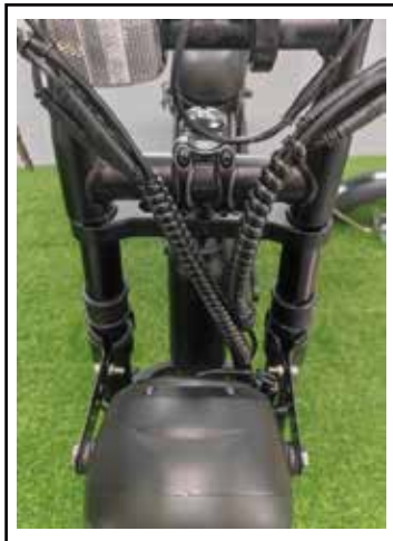
10. Install the front and tighten all the screws
